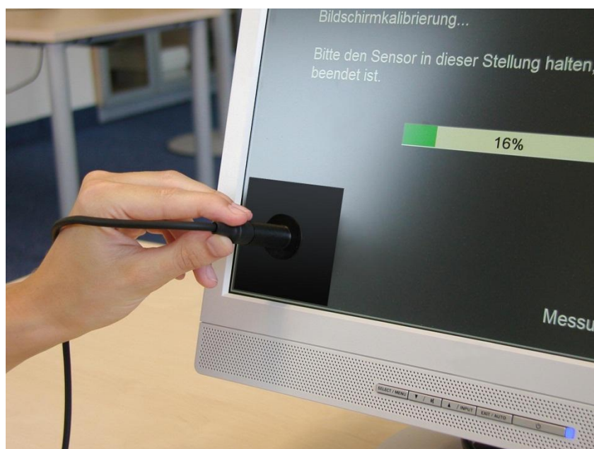
Fig. 5: Calibrating a monitor with the calibration device. The VTS workstation should be calibrated every six months and whenever changes are made to the hardware (e.g. new monitor).
