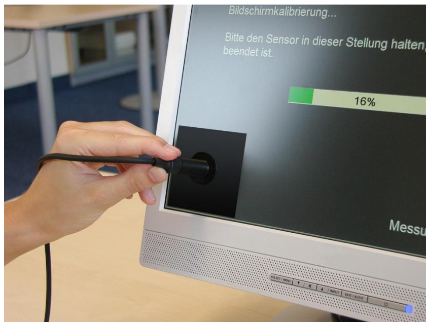
Figure 5: Calibrating a monitor with the calibration device. The VTS workstation should be calibrated every six months and whenever changes are made to the hardware (e.g. new monitor).
